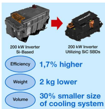
Figure 4: Improvement of performance and size reduction in power train inverter with SiC SBD technology for Formula-E racing car
