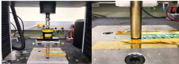
Figure 27: Pressure test instrument. The tester head lowers to the backside of the devices using a constant loading speed of 0.6 mm/min until the predetermined force is sensed by the gauge. The DUTs are surface mounted on a FR4 test coupon that is secured on the testing stage.
